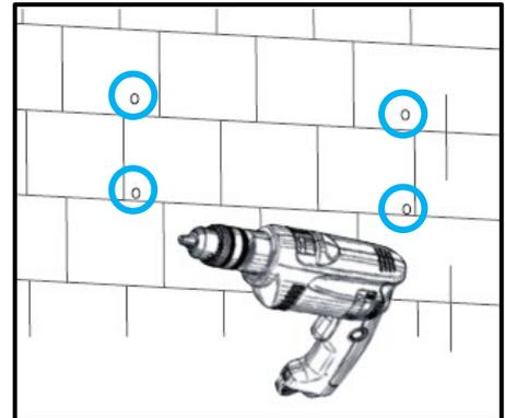
4. For concrete or brick installation, insert the expansion bolts into the drilled holes. Install the bracket to the wall, ensuring the arrow is pointing up. Use the corresponding nuts and washers (packaged together with the expansion bolts) to affix the bracket to the wall. For stud wall installation, use the proper screws and affix the bracket to the wall.
