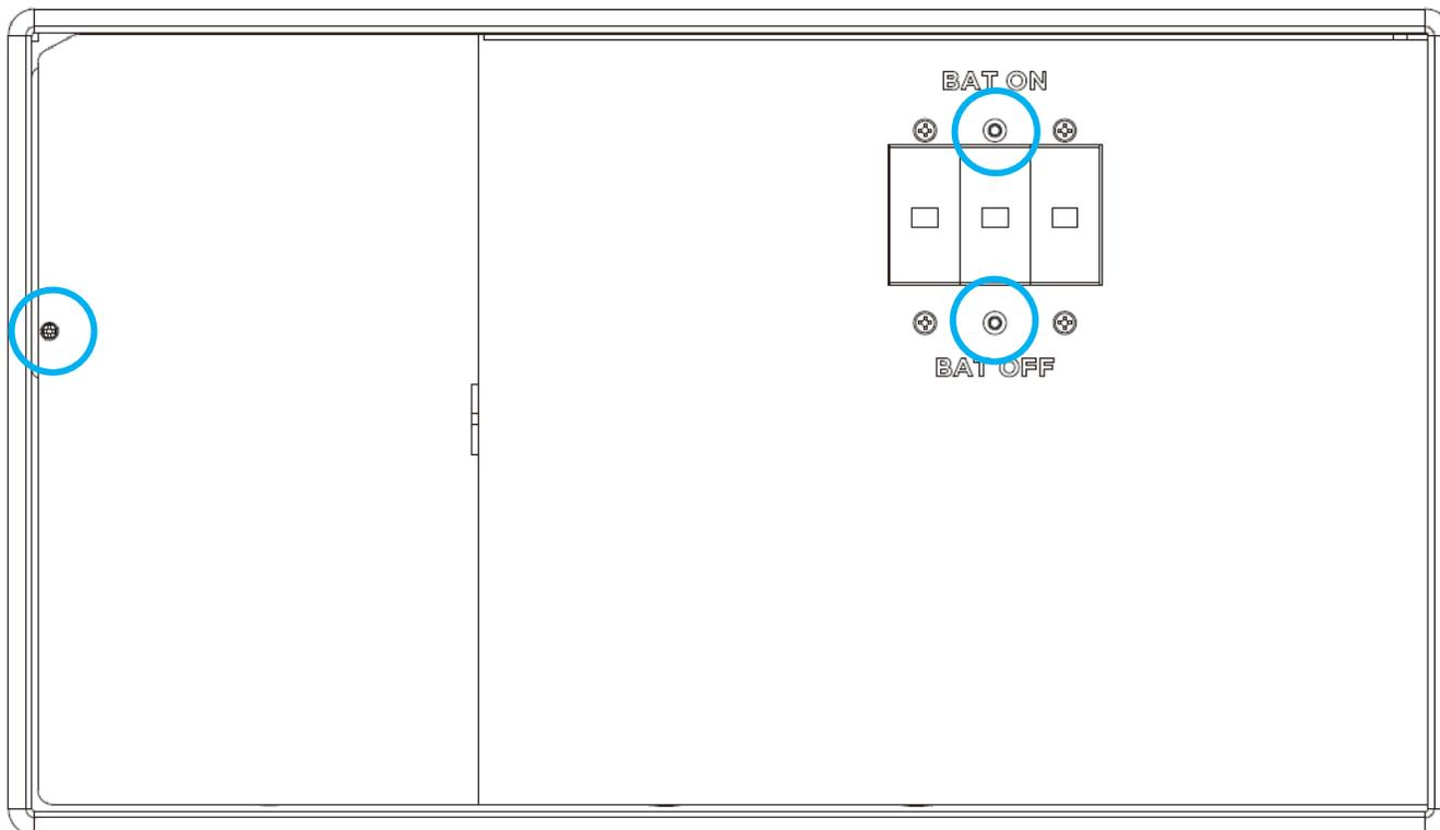
Once the cover is open, follow the sections below for connecting the wiring for PV, battery, AC, paralleled inverters, and rapid shutdown. Before connecting any wiring to the inverter, verify each wire is not carrying voltage using a multimeter.
