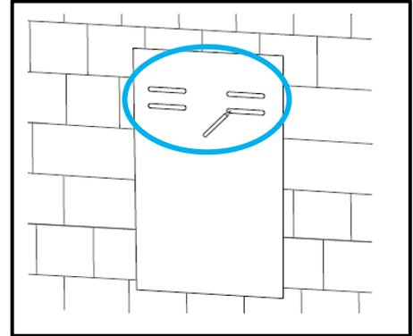
3. When installing the bracket to concrete or brick, drill 5/16 in. (8 mm) diameter holes on the marks, making sure the holes are deeper than 2 in. (50 mm) when using the included expansion bolts.
