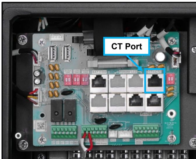
Refer to the connection diagram to the right for the correct position of the CTs. Clamp the 2 CTs onto the L1 and L2 wires at the service entry point in the main service panel as close to the meter base as possible.
