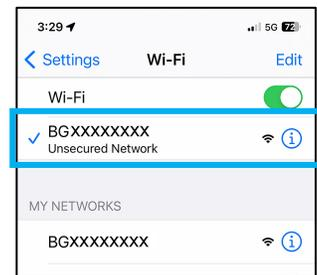
2. Once the dongle is properly configured, it should successfully connect to the home Wi-Fi network and then to the internet. The Cloud LED will illuminate once the dongle connects to the monitoring server via the internet.
